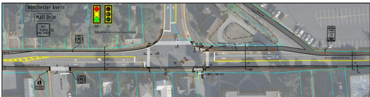
Figure 12: Winchester Avenue and Mall Drive Intersection Improvements
