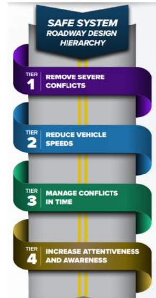
FIGURE 1. SAFE SYSTEM ROADWAY DESIGN HIERARCHY. SOURCE:
