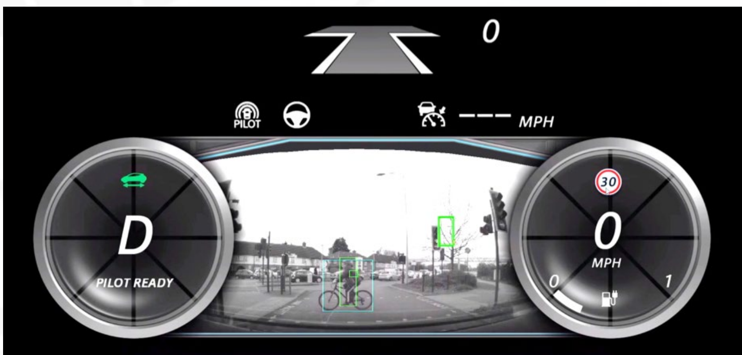
Today's semi-autonomous vehicles, like the Nissan Leaf (above), use sensors and cameras to detect traffic signals, other vehicles, pedestrians, and cyclists. Source: Fully Charged, YouTube, March 30, 2017
