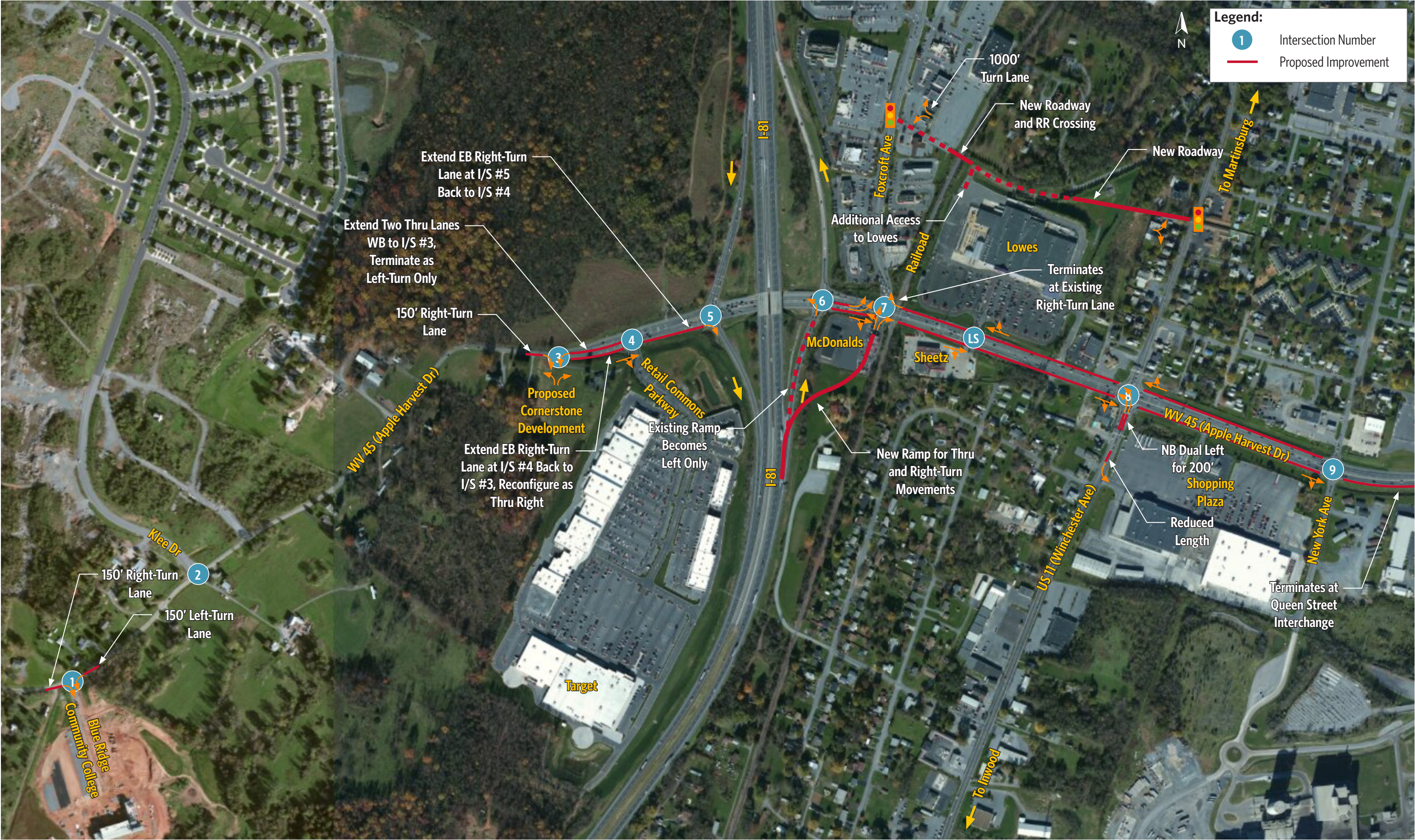
Figure 5-8: 2024 Build Alternative 4 Improvements - Ultimate Build
