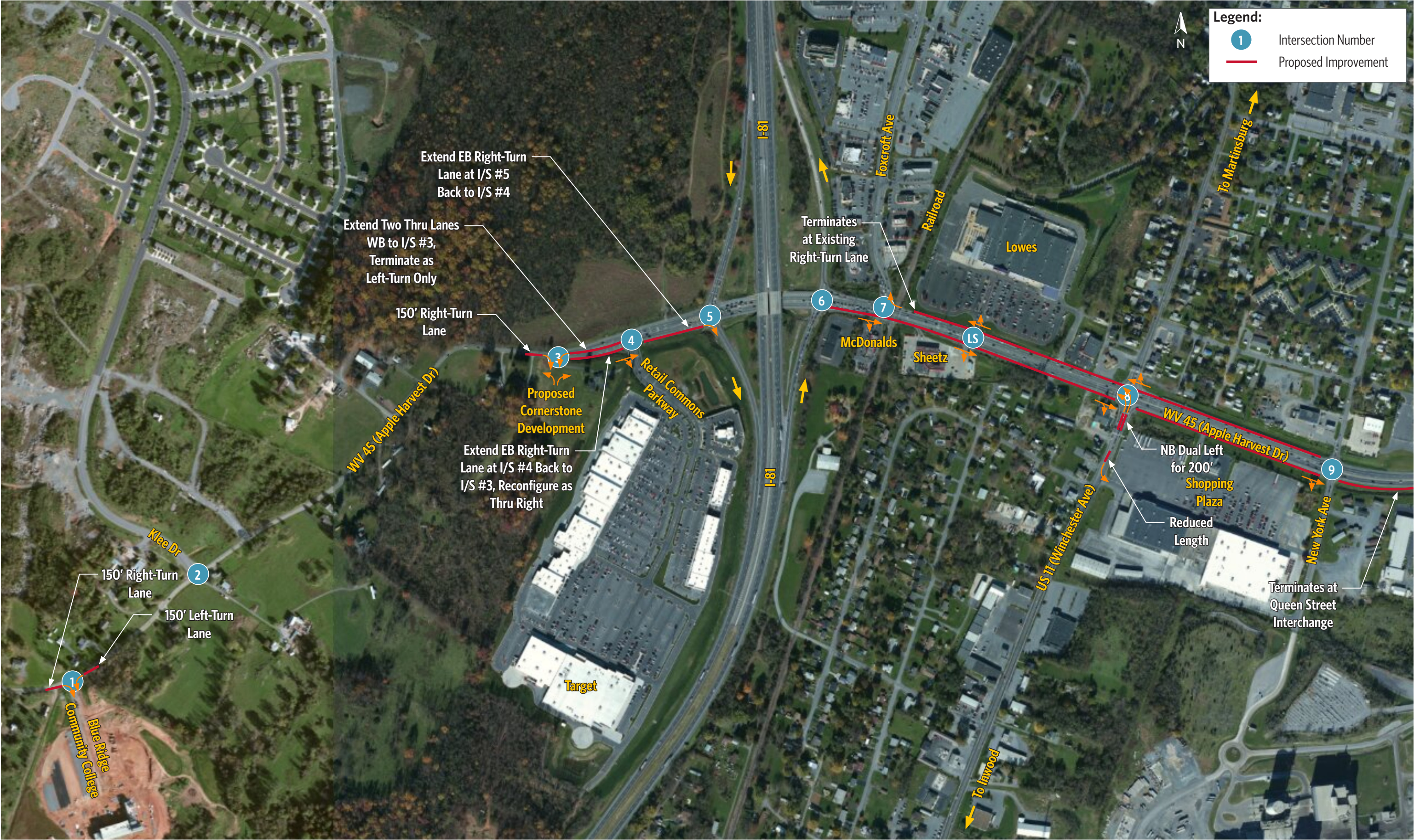
Figure 5-3: Alternative 2 Improvements - Additional Thru Capacity
