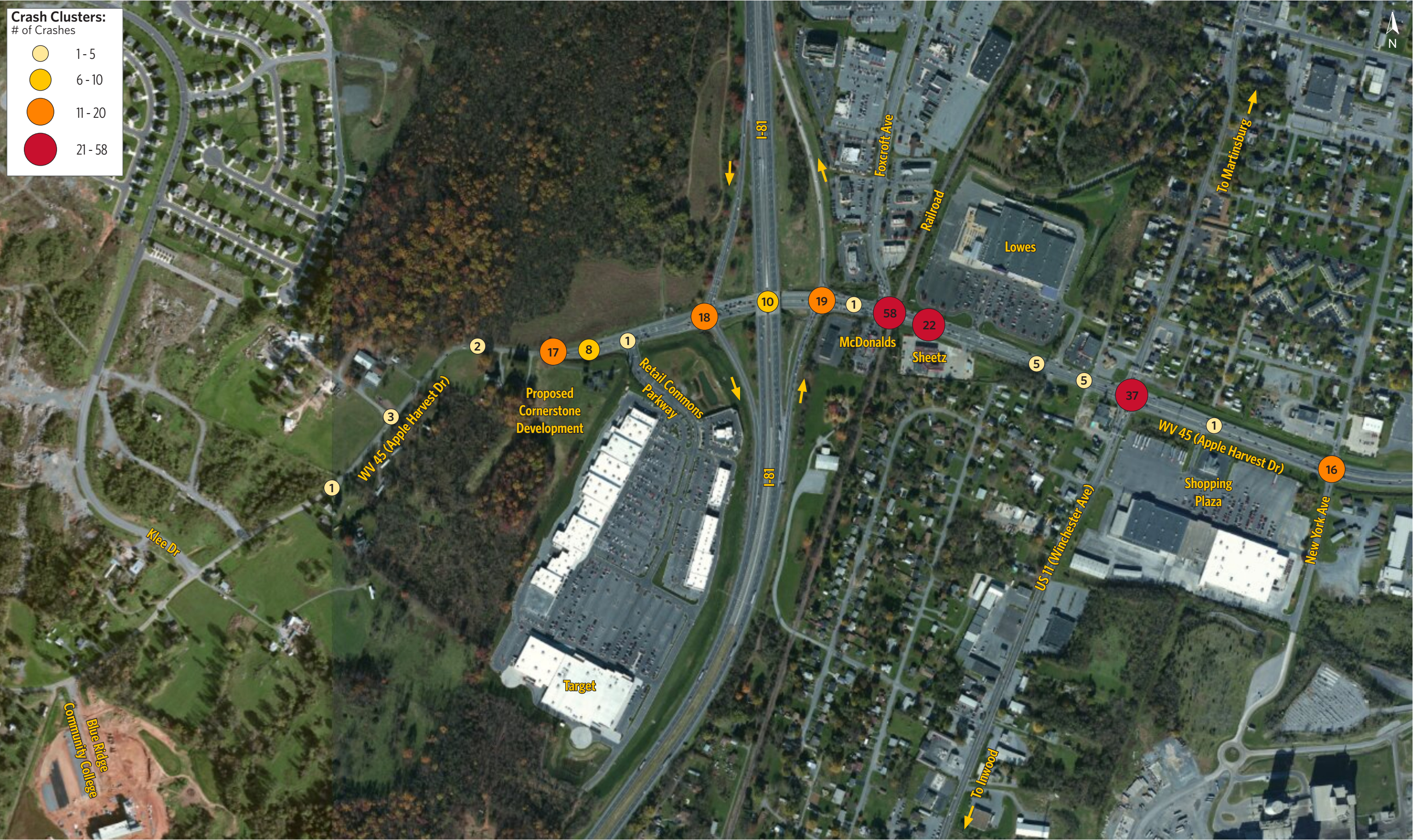
Figure 3-1: WV 45 Crash Intensity Diagram
