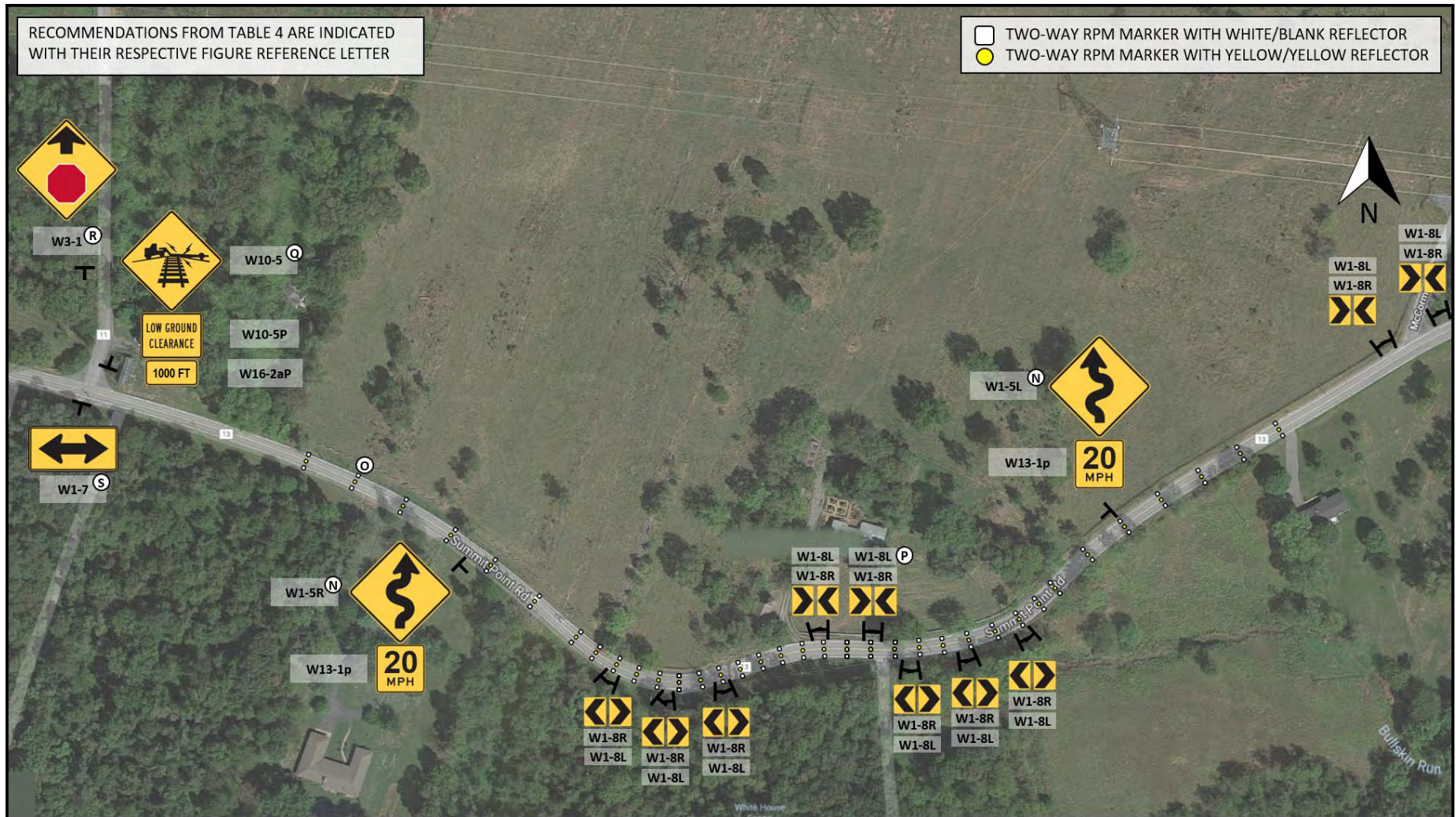
Figure 8: Signing and Pavement Marking Recommendations through Winding/Rolling Section adjacent to White House Farm
