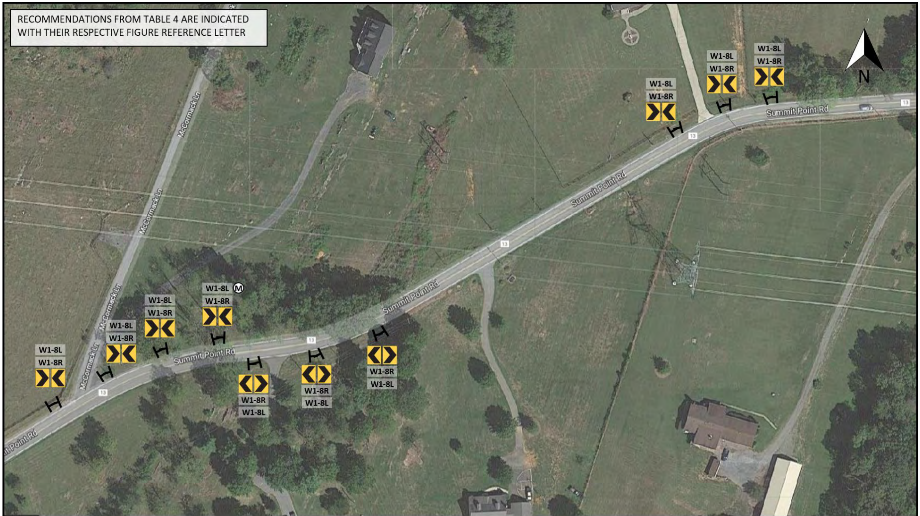
Figure 7: Signing and Pavement Marking Recommendations West of the School to McCormack Lane
