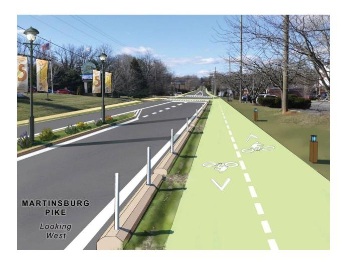
A suggested improvement, illustrated here, would include a concrete curb with rounded or angled edges to provide a solid barrier between the drive lane and multimodal path.
