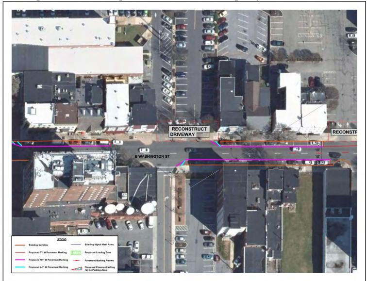
Figure 9: Pavement Marking Recommendations east of Washington St/Potomac St Intersection
