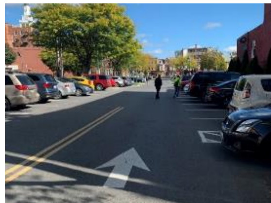
Centerline striping in the Central Lot may result in higher vehicles speeds.
