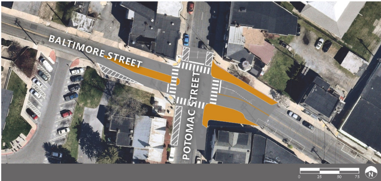
Extending the curb and reducing the crossing distance will improve pedestrian safety and visibility.
