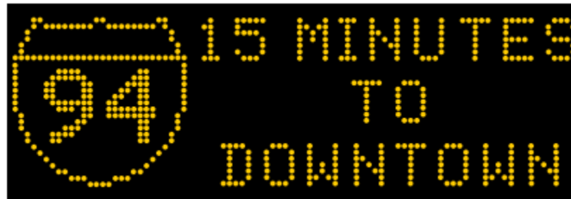
Figure 35: Low Resolution, Amber (66mm)
